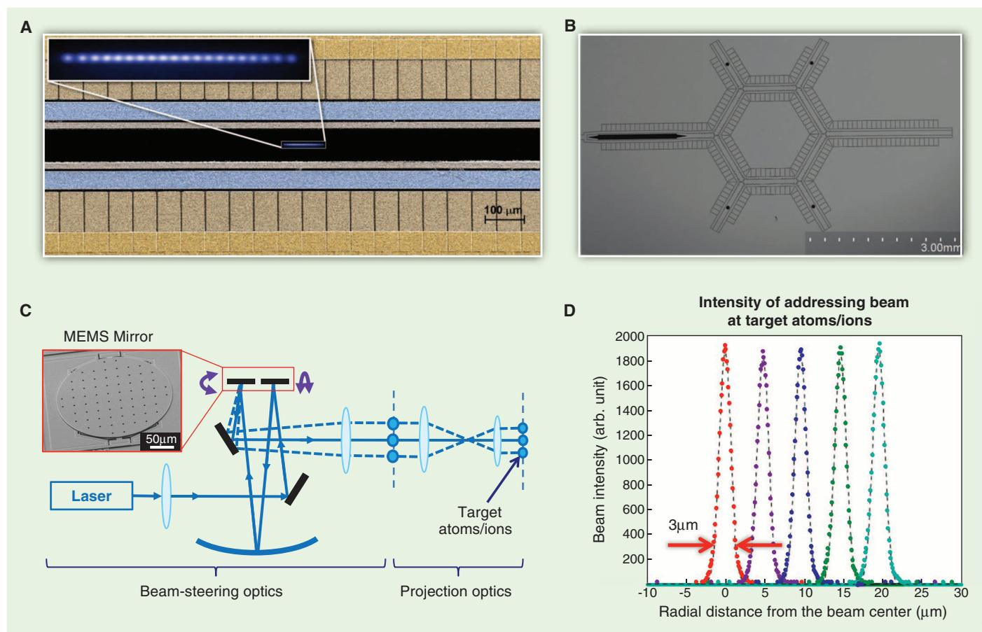
**Fig. 3.** (A) Scanning electron micrograph of a microfabricated linear trap with a long slot, with superimposed image of 20-ion chain in an anharmonic well (inset). The blue rails are RF electrodes and the rest are segments of static electrodes. [Courtesy GTRI] (B) Circulator trap with six junctions and two linear sections on either side for qubit manipulation. The other four short sections can be used as loading zones (of multiple ion species, if necessary), and the six junctions enable
